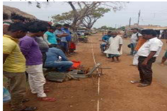
Resistivity survey at Indpur
