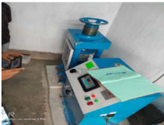
7 days Compressive strength test of M25 grade of Concrete at Package- 03 Laboratory
